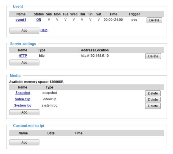
When the Event Status is <u>ON</u>, the event configuration above is triggered by motion detection, the Network Camera will automatically send snapshots via e-mail.
