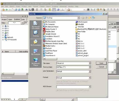
9. Save the edit using the ".crt" extension, using a file name like "CAcert.crt."
