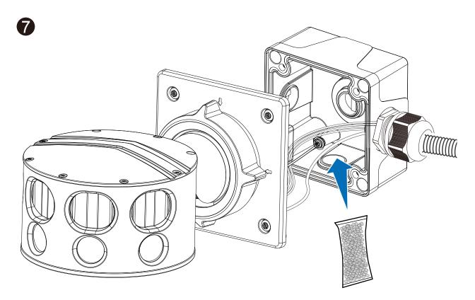
8. Secure the camera to the junction box using a T25 L-wrench. Tighten the screws.
