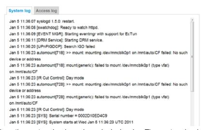
This column displays the system log in a chronological order. The system log is stored in the Network Camera's buffer area and will be overwritten when reaching a certain limit.
