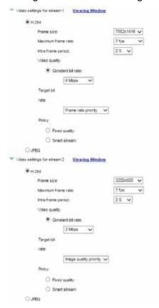
This Network Camera offers real-time H.264 and MJPEG compression standards (Triple Codec) for real-time viewing. If the H.264 mode is selected, the video is streamed via RTSP protocol. There are several parameters through which you can adjust the video performance:
