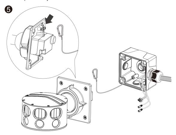
6. Install a MicroSD card. Connect the Ethernet cable and the DI/DO, audio input/output, and/or the AC 24V input (if preferred).
