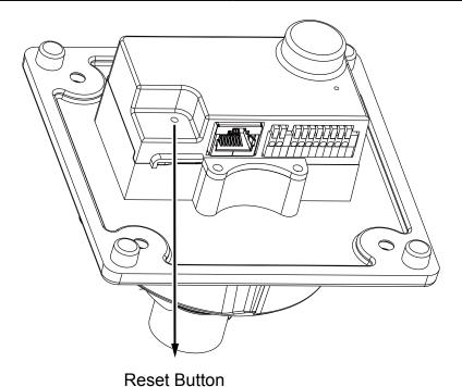
The reset button is used to reset the system or restore the factory default settings. Sometimes resetting the system can return the camera to normal operation. If the system problems remain after reset, restore the factory settings and install again.
