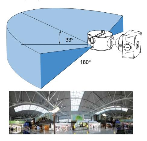
The field of view is illustrated above. Note that the higher the camera is installed, the larger is the blind spot area underneath the camera. The camera can be mounted at a height of 5 meters or higher to cover a panoramic view area with its center of view aiming at the horizon.
