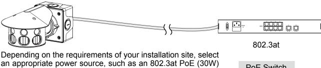
an appropriate power source, such as an 802.3at PoE (30W) for operating temperature higher than -10°C. For extremely low temperature, you will need a power source higher than 35W, such as 24V AC.
