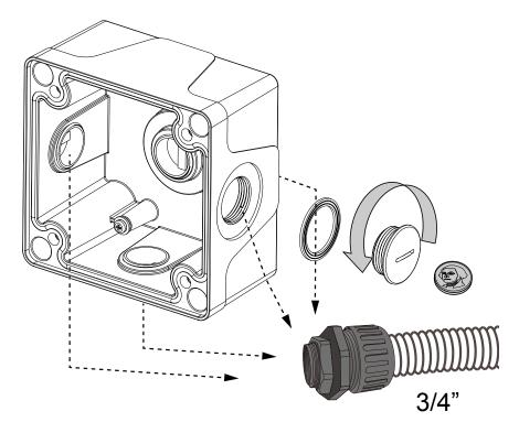
4. Route cables through the routing hole or the conduit.
