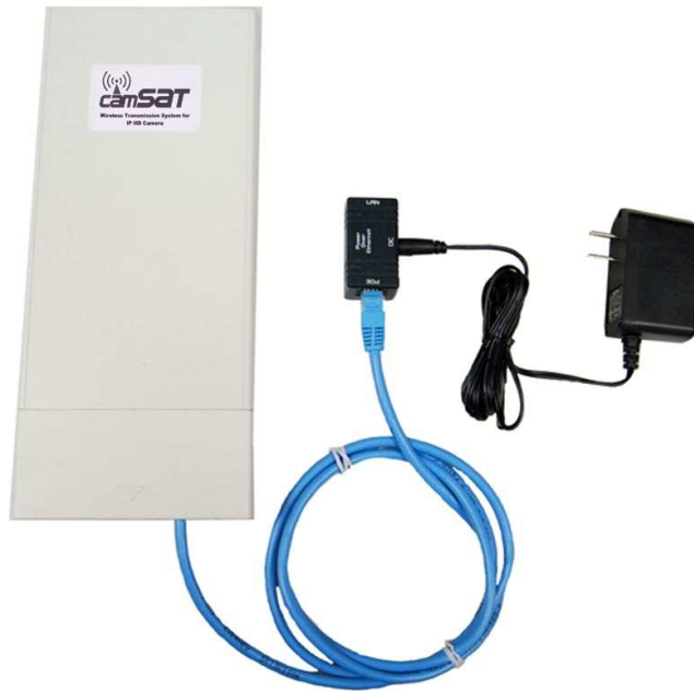
Figure 5 Plug the Ethernet cable to the RJ-45 jack of the injector
