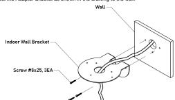
Make sure the cables are led freely through the Bracket as shown in the previous drawing and that all screws are fixed tightly. Connect the Dome Camera to the Wall Bracket as shown in the following drawing.
